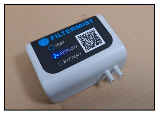
If a blue light is flashing, this means the monitor is uncalibrated. If you have attempted to calibrate, then it did not recognise the airflow. You will need to recalibrate.
