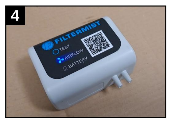
Both airflow and battery lights will flash twice when starting. After this, a continuous blue flash from the airflow light will occur. This will show that the unit is uncalibrated.
