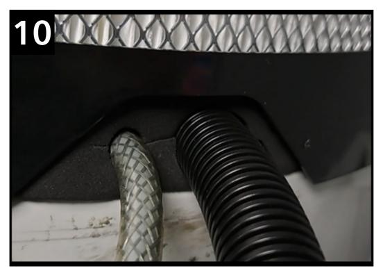
Feed the conduit through the afterfilter seal (if afterfilter is present) and secure the afterfilter into position using the clips.
