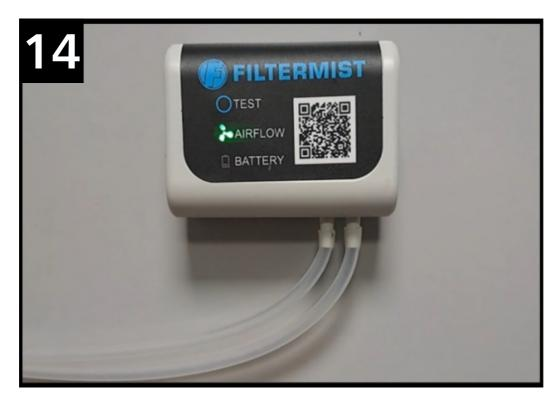
Re-fit the back cover. After two minutes the green light will revert to a flash and sense every 10 minutes.
