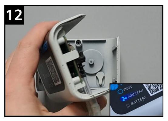
Remove the two screws on the back of the F Monitor Essential. Then remove the back cover, insert the batteries, and a double white flash on the airflow and battery lights will occur. A blue light will then flash on the front airflow light. Check that the hoses are connected inside the monitor.
