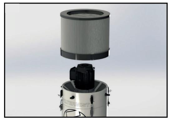
Make sure the afterfilter is not blocked by removing it from the Filtermist unit and checking.
