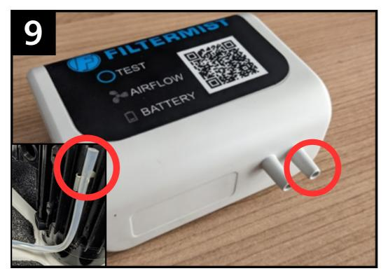
Connect the other hose to the motor using the motor clip with the hose pointing up. Then fix to the right hand nozzle on the bottom of the monitor.
