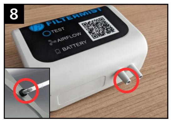
Connect the hose marked with pen to the nozzle on the diaphragm. Then connect to the left hand nozzle on the bottom of the monitor.
