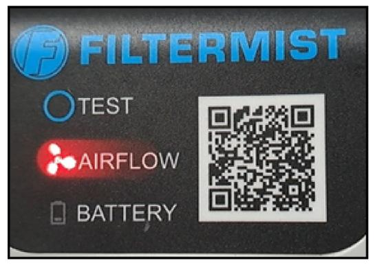
If the light turns red, check for a blockage in the air stream. See steps below.
